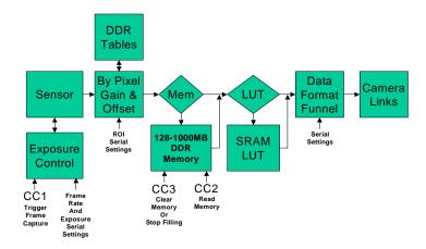
DDR Memory can be organized as a FIFO or as a circular buffer. CC3 is used to clear the memory (FIFO) or stop filling the memory (circular buffer). CC2 is used to read the top most image from memory (FIFO) or to read the oldest non-read image from memory (Circular buffer).
